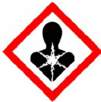
GHS 08 Carcinogenic, Respiratory Sensitizer, Reproductive toxicity, Mutagenicity, Target organ toxicity, Aspiration toxicity
